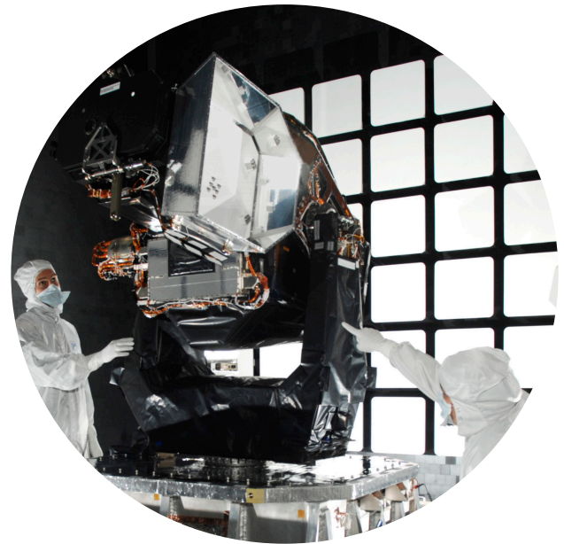
Testing of the SBSS gimbal at Ball Aerospace
