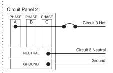
In the three-circuit, separate neutral schematic, circuits 1 and 2 are distributed from two different phases from the first circuit panel. Each circuit is supported with its own neutral and a common ground. Circuit 3 is distributed from the second circuit panel and is supported by its own neutral and ground.
