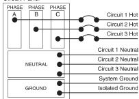
On a single 3-phase circuit panel, three circuits are distributed as shown.
